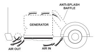
Figure 2.13 - Air Inlet in Vehicle Skirt
